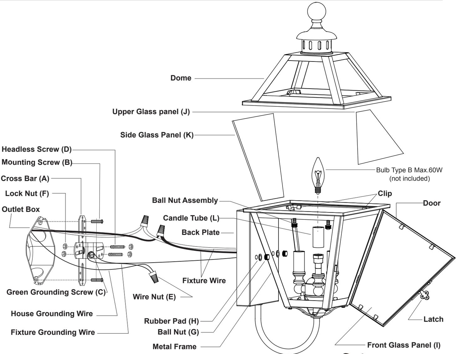
1. Take a side glass panel and gently place the side glass panel into the metal frame in place, then pressing the clips of the metal frame to secure the side glass panel. (See Fig. 1)
