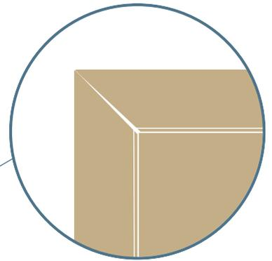
When wood shrinks, miter joints open as shown above.
